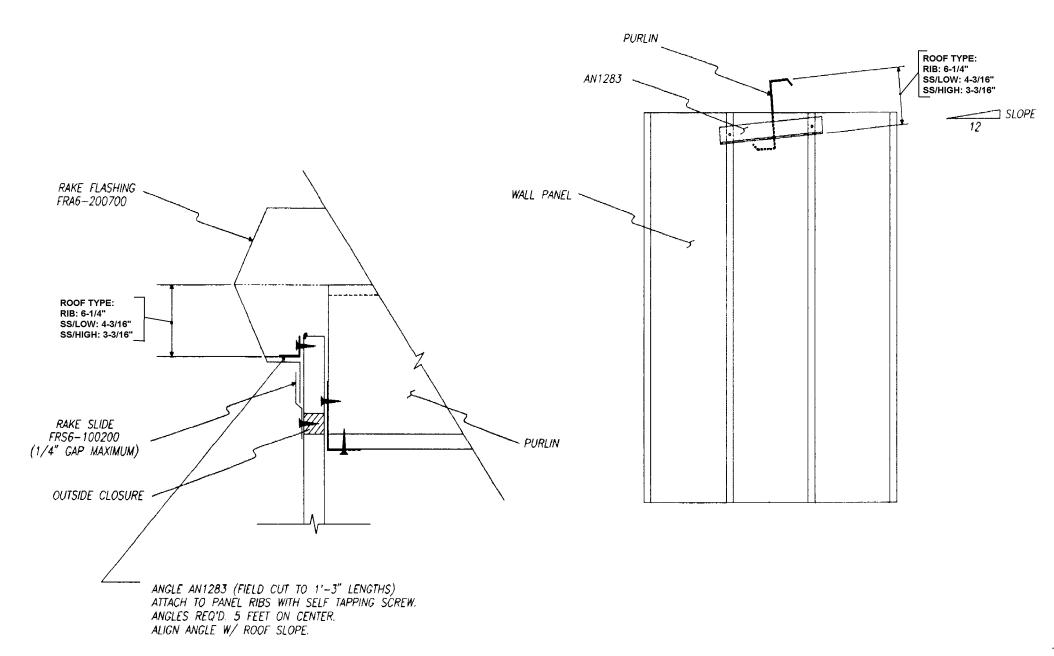
NOTE: RETAINER ANGLES ARE TO KEEP RAKE FLASHING FROM BECOMING DISENGAGED FROM THE RAKE SLIDE IN HIGH WIND CONDITIONS.
